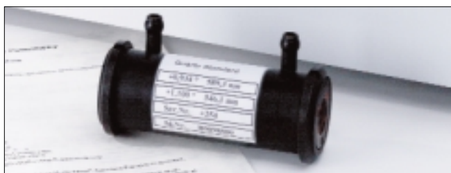
Figure 6. The quartz control plate allows GLP-compliant instrument performance verification.
