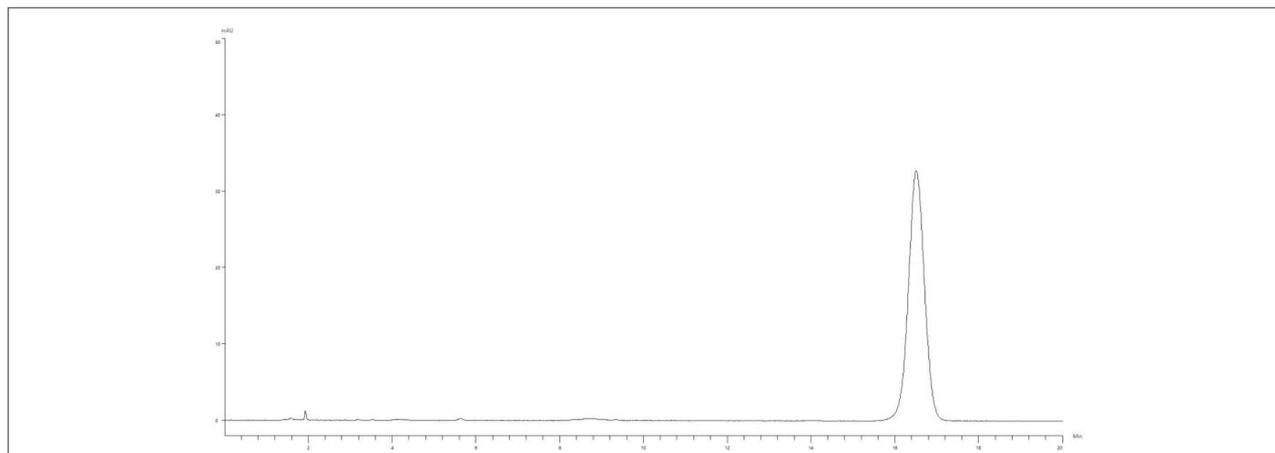
Figure 2: Analysis of amlodipine besylate using an Epic C18 column (150 x 4.6 mm, 5 µm).
