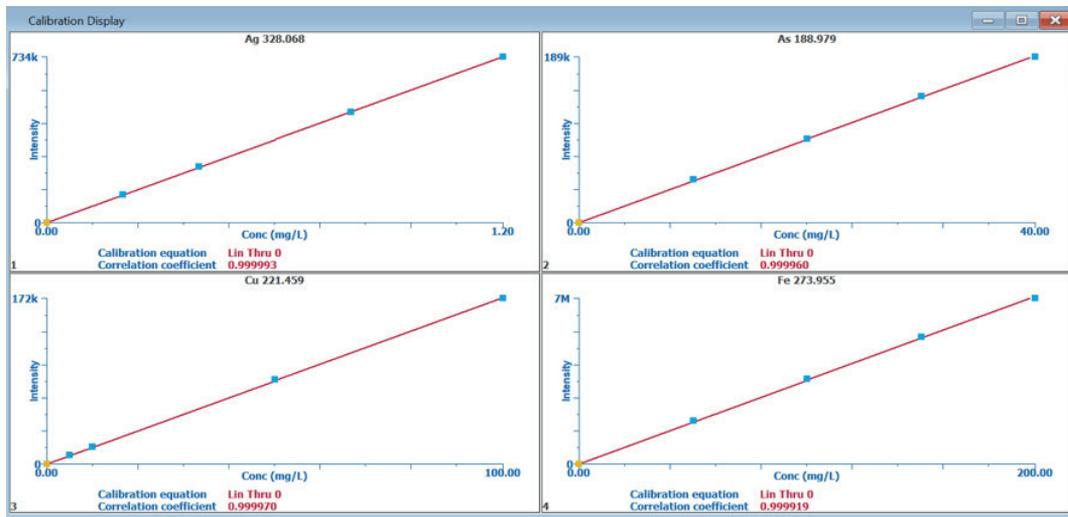
Figure 1. Calibration plots for Ag, As, Cu, Fe.
