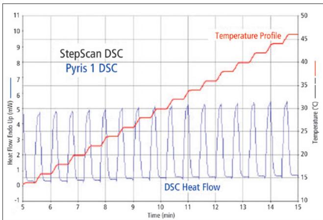
Figure 1. StepScan DSC approach using time-temperature profile.
