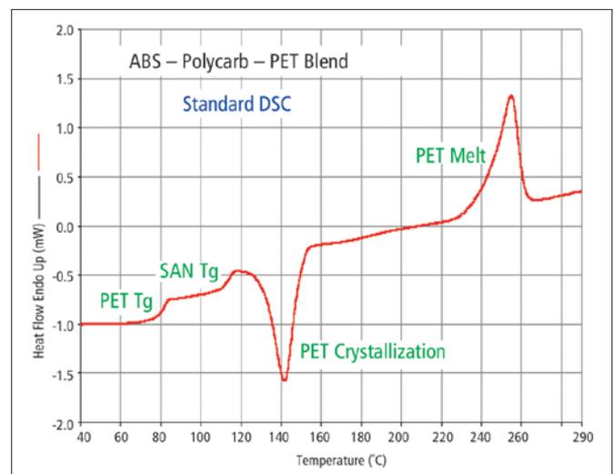
Figure 2. Standard DSC results obtained on polymer tri-blend of ABS, polycarbonate and amorphous PET.
