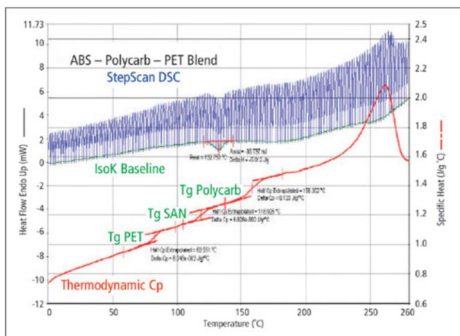
Figure 3. StepScan DSC results on polymer tri-blend.
