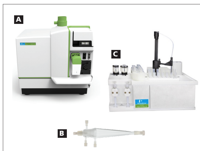
Figure 1. Hardware components for Single Cell ICP-MS: NexION 2000 ICP-MS (A), Asperon spray chamber (B), Single Cell Micro DX Autosampler (C).
