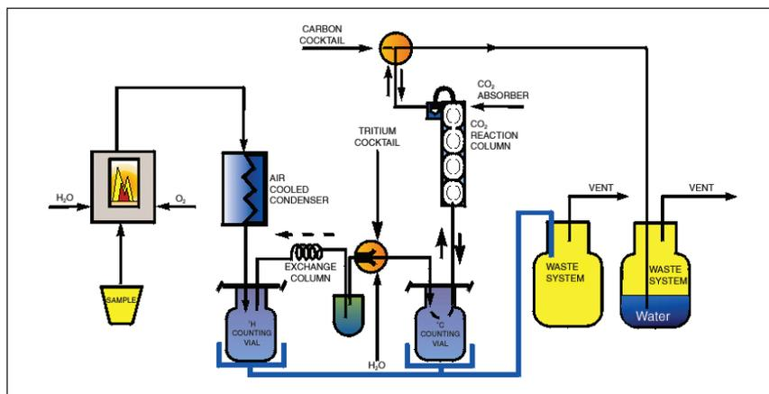
Figure 2. Non-catalytic combustion of organic samples by flame oxidation to  $^3\text{H}_2\text{O}$  and  $^{14}\text{CO}_2$ .
