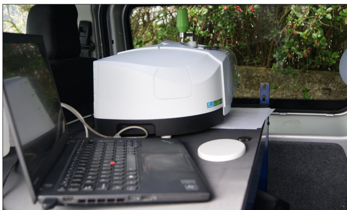
Figure 1. Compact and portable, the Spectrum Two™ FT-IR is easy to install and use within a mobile analytical vehicle.
