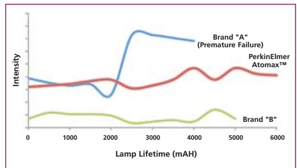
Atomax lamps demonstrate high initial intensity and minimal variation to the lamp warranty period (5,000 mAH) and beyond, comparing favorably with other AA lamps tested under the same conditions.
