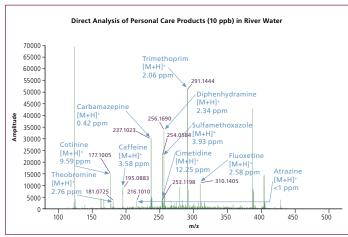
With accurate mass, the AxION DSA/TOF system records true molecular signals, presenting perfectly clear, easy-to-read data without any complicated post-processing.
