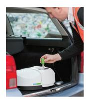
Spectrum Two incorporates a number of features to enable your infrared analysis to move out of the laboratory. Multiple power options allow Spectrum Two to be used with or without external mains power. Once powered, a fast warm-up facilitates rapid measurement while optional wireless connectivity allows portable PC control. Compact and robust, Spectrum Two can easily be transferred from one location to another and the user-install capability allows instruments to be set-up by anyone, anywhere.
