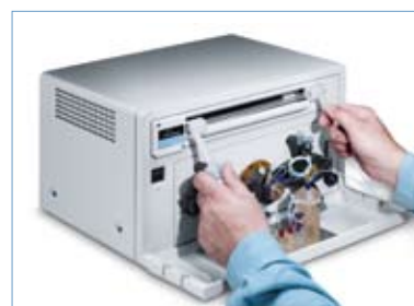
Figure 6. Easy interchange of FIMS absorption cell.
