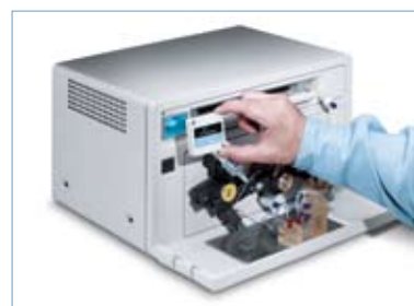
Figure 7. Quick, simple access to mercury light source.
