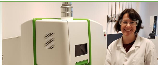
From an analytical perspective, the Avio 200 ICP-OES has extended linear range with dual viewing technology for optimal viewing. It has no limitations neither to the axial or the radial view, delivering an extended linear dynamic range which can minimize sample preparation and dilution.
