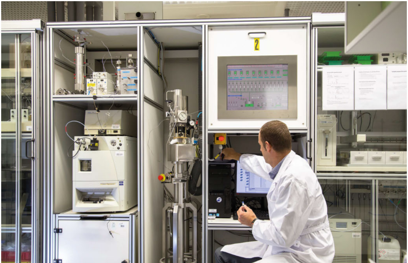
HPLC set-up with system layout (flat screen). On the left, a Waters Micromass 996 with Photo Diode Array detection.
