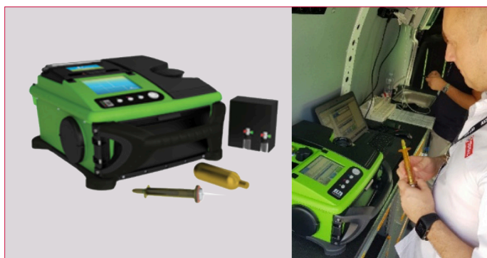
Figure 2. Compact and portable, the Torion T-9 GC/MS is easy to install and use within a mobile track-side analytical vehicle.
