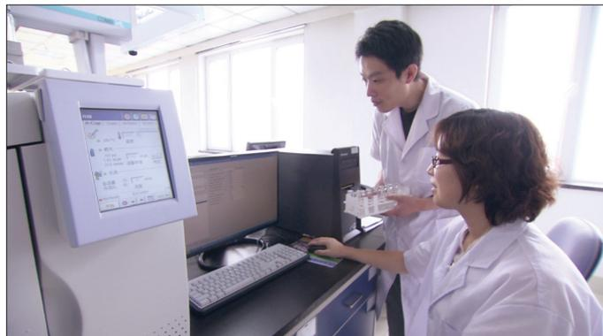
Using PerkinElmer GC/MS to analyze the fragrance of hops in beer.
