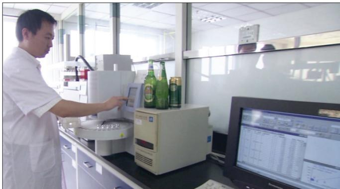
Using PerkinElmer GC-HS with PFPD detector to analyze ppt level sulfur in beer sample.
