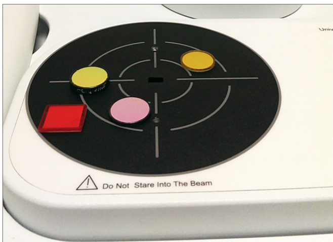
Figure 5. Sample measurement surface of the URA accessory. Using internal kinematic optics the light beam is directed to the measurement port at the center. Samples lay flat covering the port.
