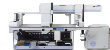
The Gripper Arm's rotational ability is used to deliver the OptiPlate™ or AlphaPlate to the EnVision Alpha reader in a JANUS-EnVision Integrated system.
