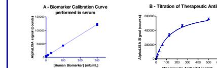
**Panel A:** The biomarker of interest was diluted in human serum and titrated in an AlphaLISA direct sandwich assay. The performance parameters of the assay were determined (e.g. LDL = 1.3 nM/mL) and found to be comparable to published ELISA assay parameters.
