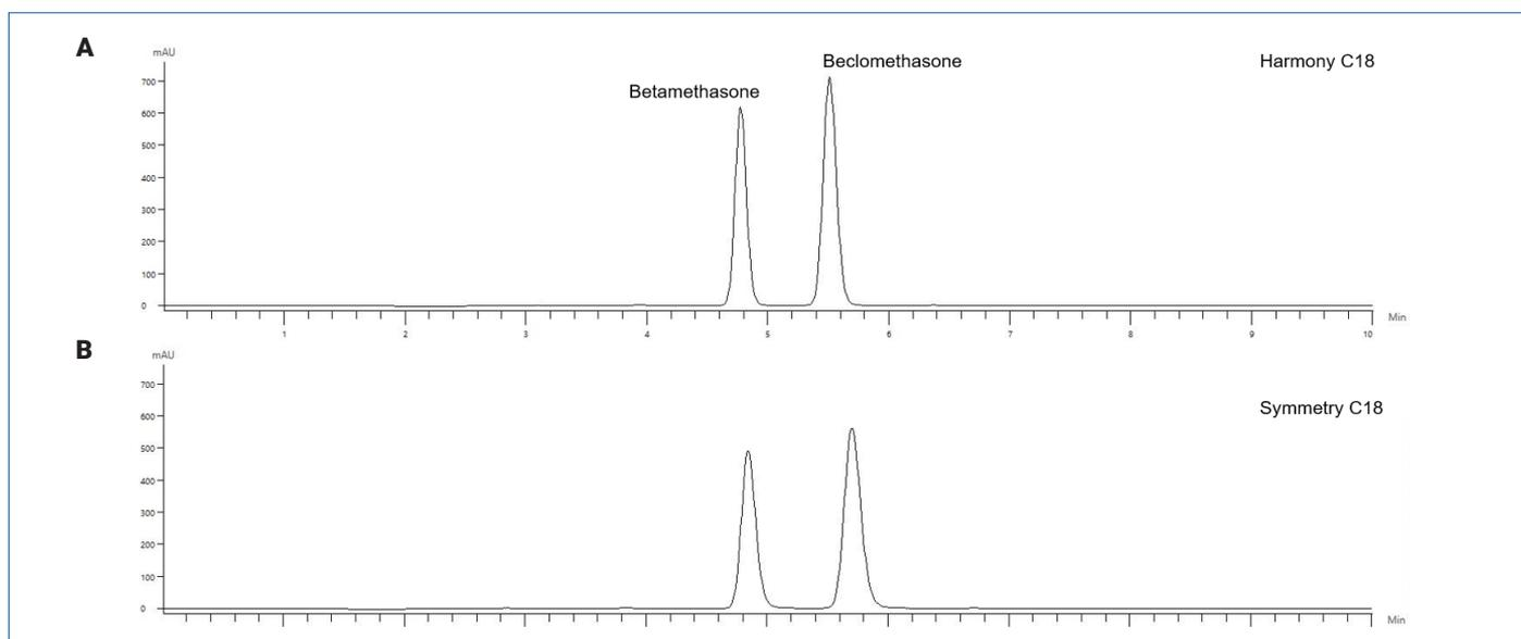
Figure 4: Analysis of betamethasone dipropionate using Harmony C18 (A) and Symmetry (B) columns.
