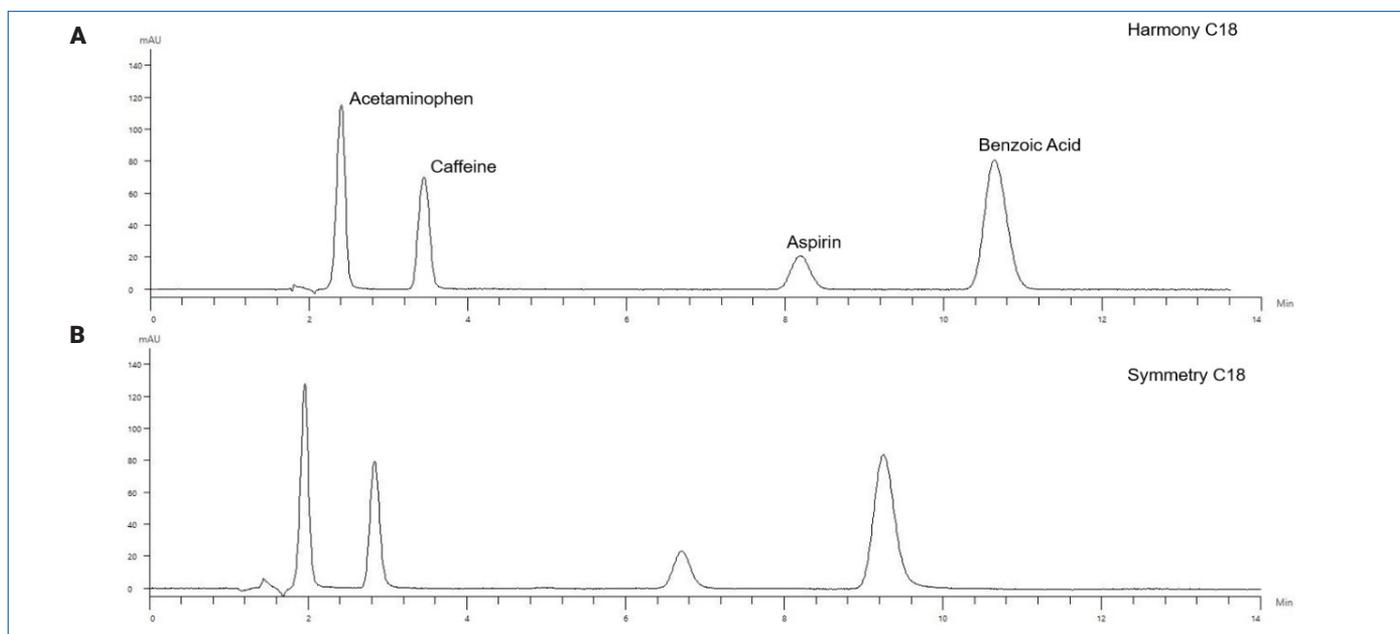
Figure 6: Analysis of acetaminophen, aspirin and caffeine using Harmony C18 (A) and Symmetry C18 (B) columns.
