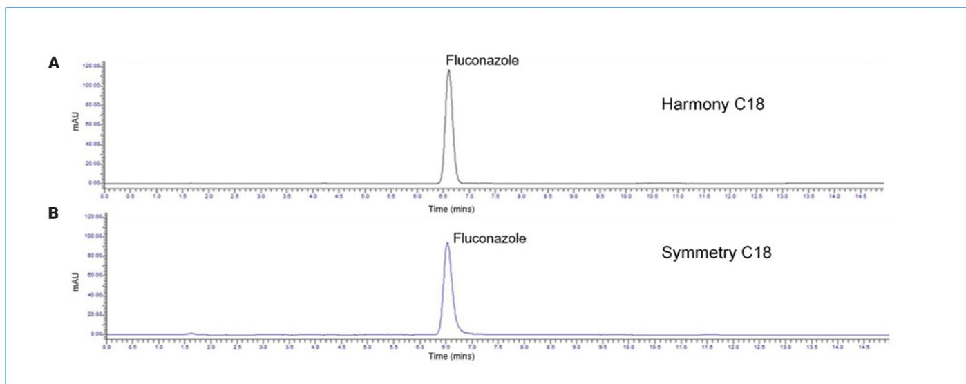
Figure 2: Analysis of fluconazole using Harmony C18 (A) and Symmetry C18 (B) columns.
