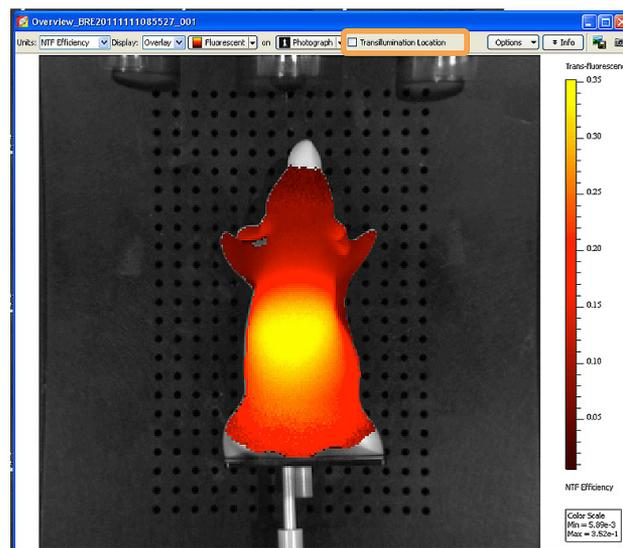
14. Switch to NTF Efficiency in the Units dropdown at the top of the image to apply the normalization and proper calibration. See Transillumination Fluorescence – Normalized Tech Note 6c for more information about NTF Efficiency.
