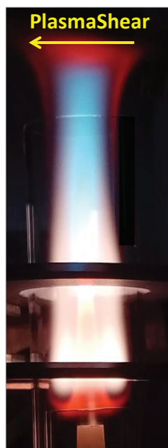
Figure 4. Inductively coupled plasma aspirating 1000 ppm Y, with the red tail plume removed with PlasmaShear.
