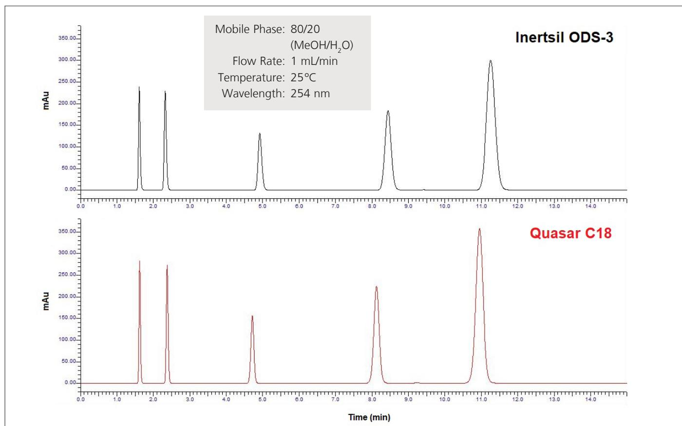
Figure 1. Chromatograms of a neutral compound test mix on Quasar C18 and Inertsil ODS-3 columns.
