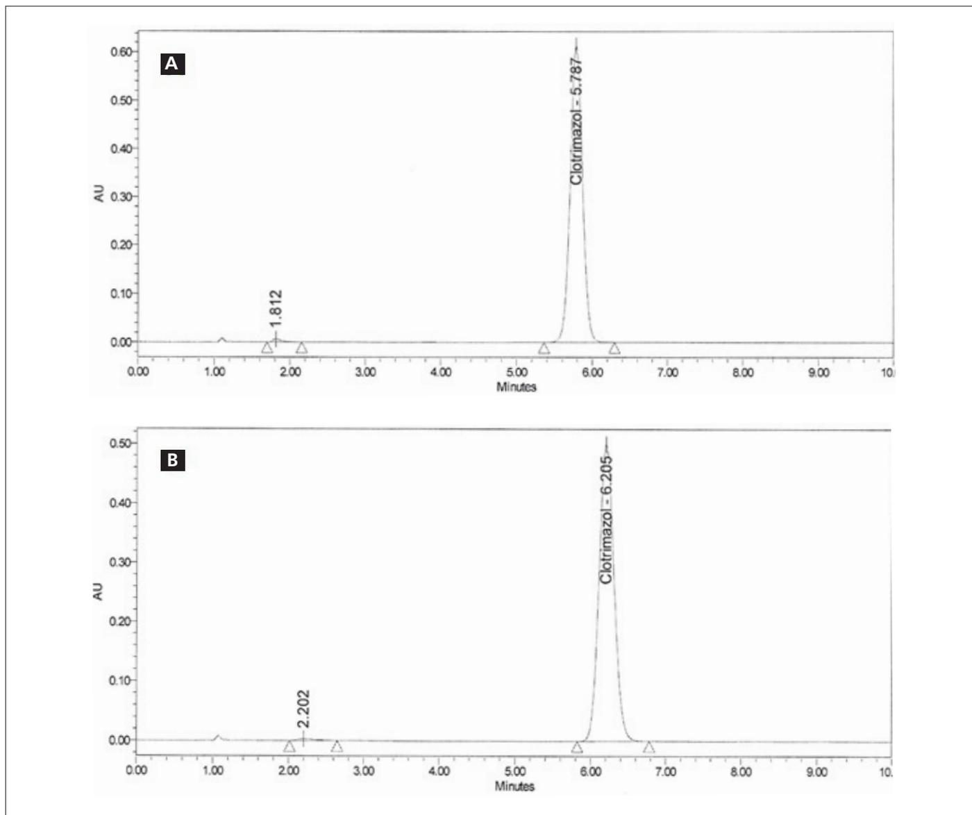
Figure 5. Analysis of clotrimazole using Quasar C18 150 x 4.6 mm, 5  $\mu$ m (A) and Inertsil ODS-3 150 x 4.6 mm, 5  $\mu$ m (B).
