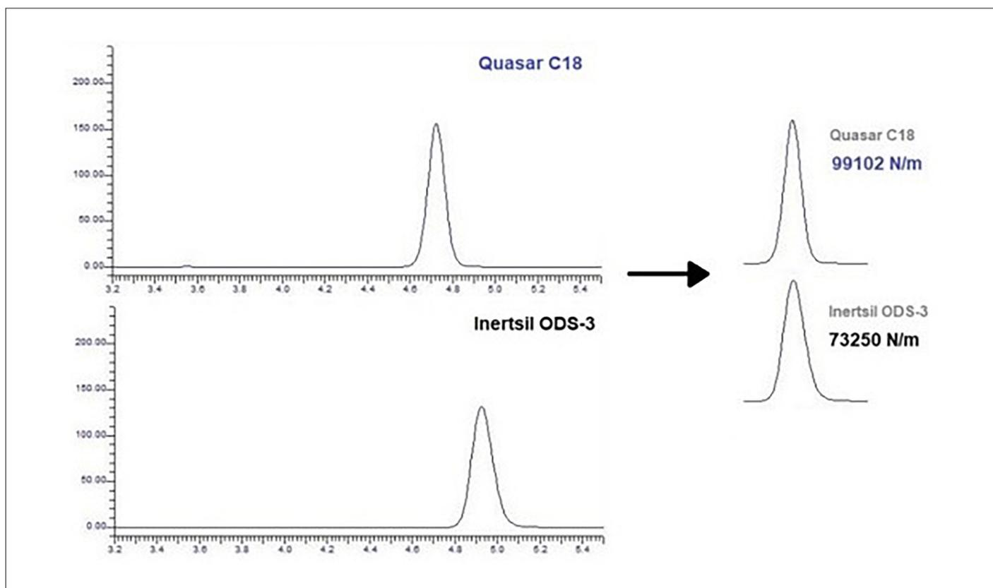
Figure 2. Toluene peak obtained using Quasar C18 and Inertsil ODS-3.
