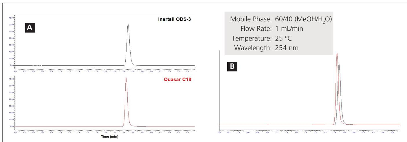
Figure 3. A) pyridine peak obtained using Quasar C18 (red) and Inertsil ODS-3 (black) columns. B) Overlay of pyridine peaks on Quasar C18 (red) and Inertsil ODS-3 (black).
