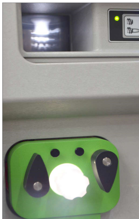
Figure 8. NexION 2000 ICP-MS with stable plasma operating with its back open to air.
