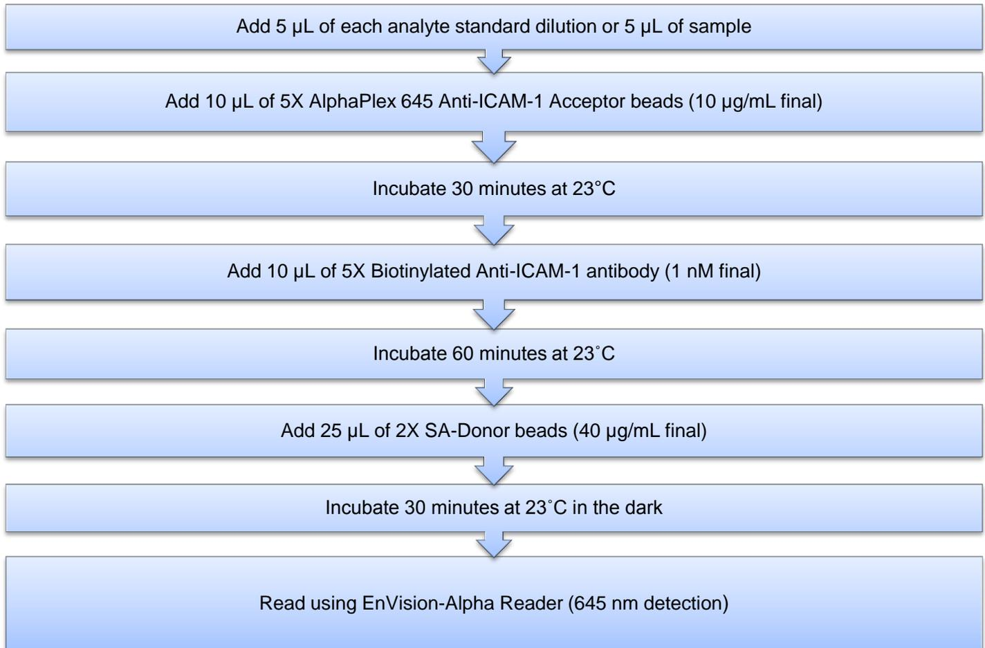
**Read Settings:** AlphaPlex 645 signal is detected using an EnVision Multilabel Reader equipped with the Alpha option using the following settings: Total Measurement Time: 1000 ms, Laser 680 nm Excitation Time: 180 ms, Mirror: 670as (Barcode# 605), Emission Filter: Wavelength 570nm, bandwidth: 100nm, Transmittance 75%, (Barcode# 244).
