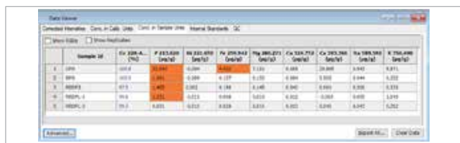
Figure 4. Syngistix software's Data Viewer automatically highlighting samples which are above user-defined thresholds.
