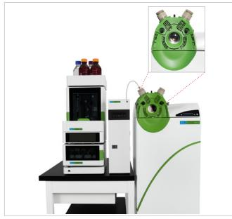
Figure 1: Picture of the source area of the QSight LC/MS/MS where two separate ionization probes are shown.
