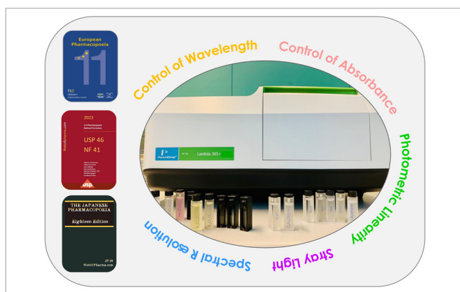
Figure 2. Lambda 365+ UV/Vis Spectrophotometer with the CRM standards used for the Operational Qualification. Image source: www.pharmasopworld.com/ .
