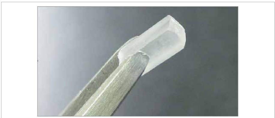
Figure 4. Example of a polymer sample cut to have a flat top and bottom, for measurement by both DSC and FTIR.
