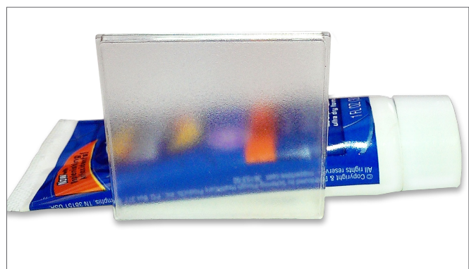
Figure 2. Pictured against a small tube of commercial sunscreen is the recommended PMMA substrate for SPF testing, the HELIOPATE HD 6 (50 mm x 50 mm, 6 microns).
