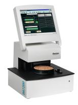
During this time approximately 300 full spectra are collected and averaged. Since the sample is analyzed in an open dish, the problems associated with sample
