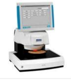
As the samples are analyzed in reflectance NIR spectroscopy from above in open dishes, the problems associated with unclean sample cups are avoided and operator influence on results is minimal.
