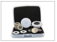
DescriptionPart No.2500 Run Kit for High Pressure 100 mL (100 Bar) Digestion VesselsN3133024Consumables for approximately 2500 digestions with High Pressure 100 mL (100 Bar) Digestion VesselsIncludes 10 Pressure Seals (N3133023), 7 Rupture Cap Discs (N3133022),50 PEEK Ring Nuts (N3133011), and 5 Lip Seal Rings of the Gas Containment Manifold (N3134000)
