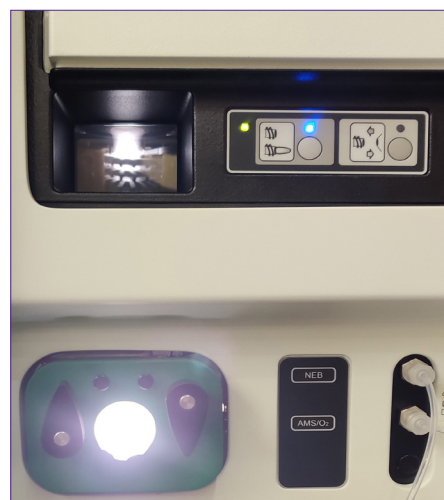
Figure 8. NexION 2200 ICP-MS with stable plasma operating with its back open to air.
