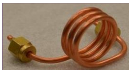
Figure 3. Copper load coil used in most ICP sources.
