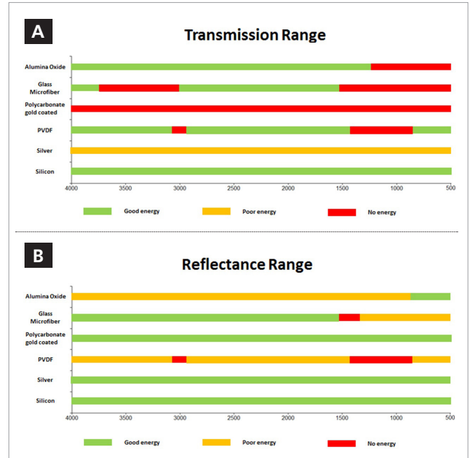
Figures 2a and 2b. Transmission and Reflectance ranges of filter types.
